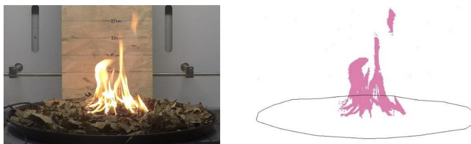
Fig. 32 Flame area during the fire test 1 in time of 20 s
